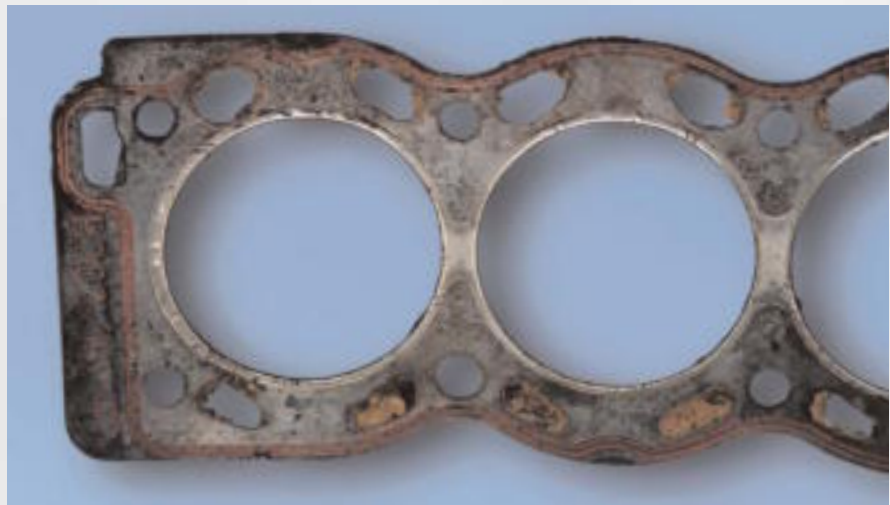
Failed cylinder-head gasket
